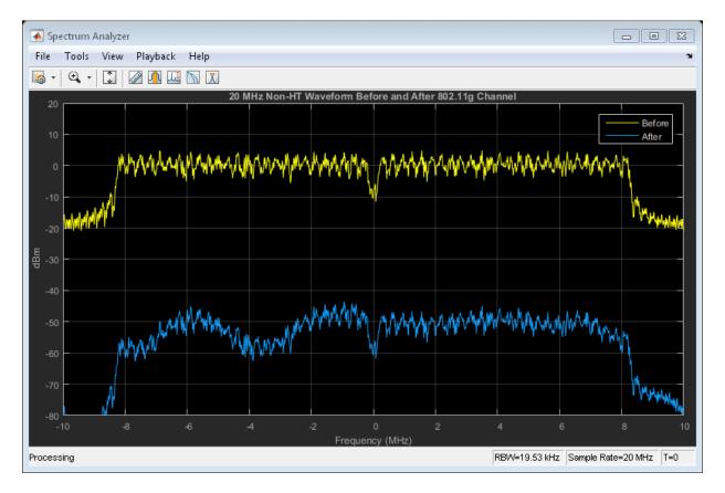
The free-space path loss accounts for the approximatley 50 dB of separation between the waveform before and after it passes through the 802.11g channel.
