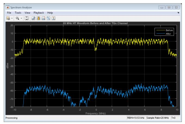
The path loss results from the default transmitter-to-receiver distance of three meters, and from shadowing effects. This path loss accounts for the roughly 50 to 60 dB of separation between the waveform before and after passing through the TGn channel. The frequency selectivity of the delay profile is seen in the signal level variation across the frequency spectrum.
