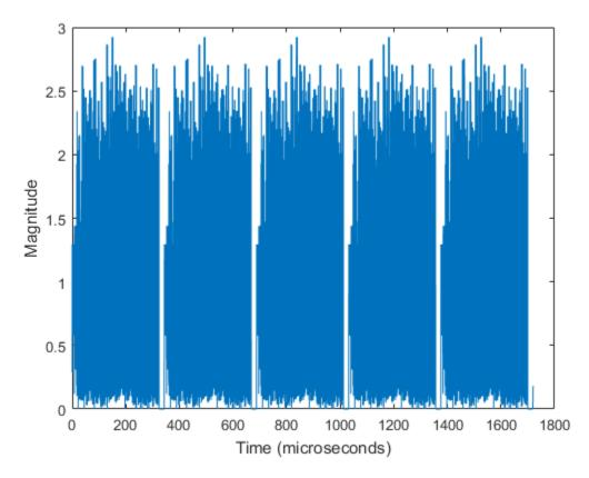
The plot shows five VHT format packets, with each packet separated by 20 microseconds of idle time.
