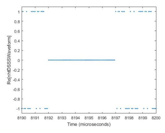
Sample values in DSSS modulation are -1 or 1. The plot shows the real values for a section of the waveform that includes the tail end of packet one, the 5 microsecond idle period, and beginning of packet two for the non-HT format DSSS modulated waveform.
