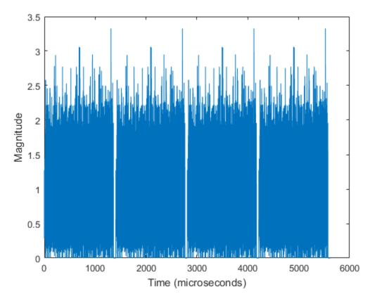
The plot shows four non-HT format OFDM modulated packets, with 45 microseconds of idle time separating each packet.
